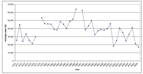
The water lost from the canal system is mostly recoverable from the groundwater. Figure 2 shows the amount lost to range from ~18,000 af in 2009 to a maximum of ~64,000 af in 1989 and on average 38,264 af of water is lost. Other data, for example, Table 3 of the 2000 Water Management Plan (http://www.archive.org/download/watermanagementp00borcrich/watermanagementp00borcrich.pdf), show that on average 28,500 af are lost to recharge each year from the District's system.
