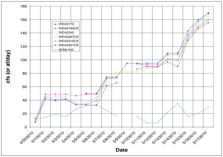
Figure 4. Screenshot showing upstream and downstream flows at two locations. The difference in flow between the green (upstream) and blue (downstream) lines is loss to groundwater.
