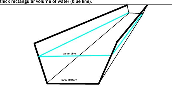
Figure 1. The top surface of the ponded canal water was modeled as a one inch thick rectangular volume of water (blue line).
