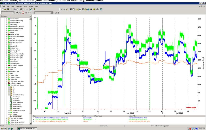
Figure 5. Losses to groundwater as measured by difference in flow between two SCADA stations. Manual overpours from STORM are measurements taken with the weir stick method.
